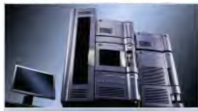
Figure 1. System configuration of Waters ACQUITY UPLC / TQD
